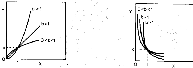
Fig. 9. Plot of the linearizable curve y=ax^b , where a,b > 0 . The linear form is \ln y = \ln a + b(\ln x) (redrawn with permission from Daniel and Wood, 1971).
