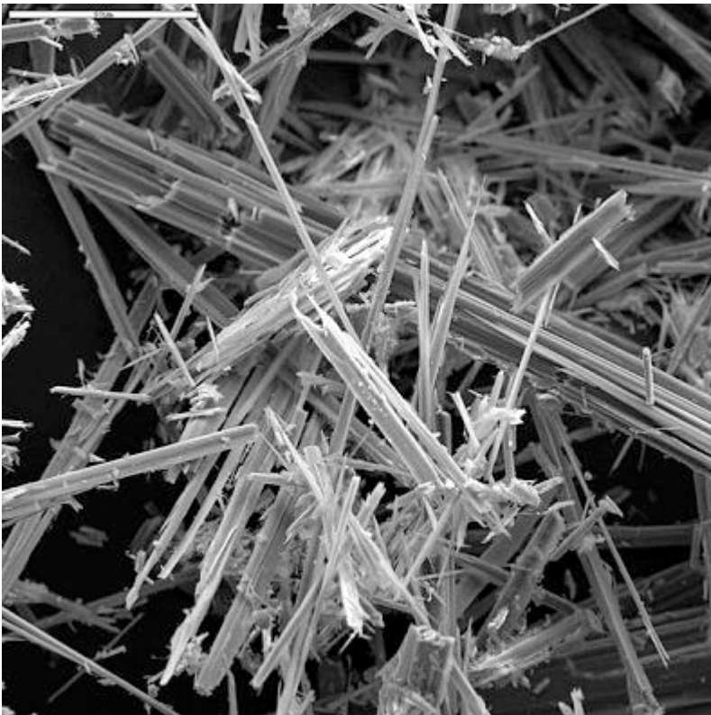
Figure 3. Asbestos fibers are small and can easily penetrate lung tissues.
